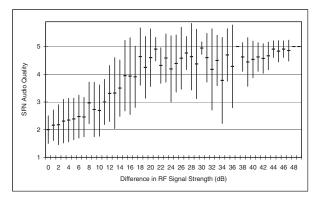
**Fig. 3:** SFN audio quality as a function of the RF field strength difference from the two transmitters
