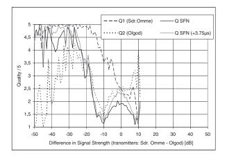
Fig. 6: Same transmitters as in fig. 5, but a different measurement route. Extra delay in the MPX signal inserted to minimize the delay difference.
