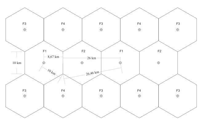
Fig. 7: Simple model of an aera covered by 4 SFN networks.
