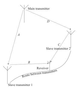
Fig. 2: Diagram showing the signal path from the main transmitter, via the slave transmitters to the receiver.
