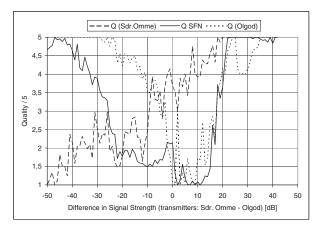
**Fig. 5:** Audio quality as function of RF signal strength difference. "Sdr. Omme" and "Olgod" are the names of the transmitters.
