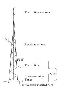
**Fig. 1:** Components of a slave transmitter site. The signals are written next to the cable. FMR is the received FM signal, FMT is the transmitted.
