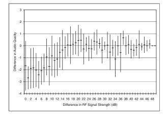
**Fig. 4:** SFN audio quality impairment a function of the RF field strength difference from the two transmitters
